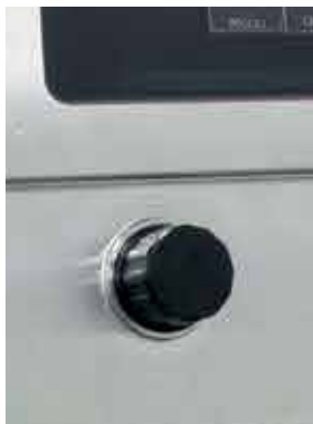
Gasketed metal cover for USB port
