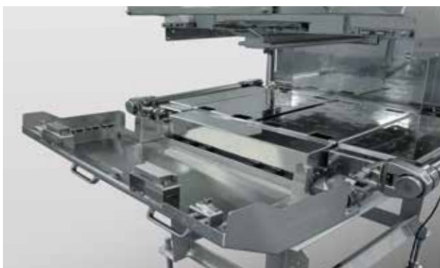
Open access to food contact area (front cover opened)
